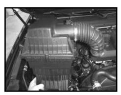
Step 4 Lift up to remove the stock air box and intake tube assembly from the vehicle.
