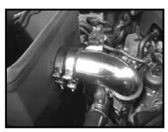
Step 11 Install the intake tube as shown and once in position tighten the clamps. Then reconnect the MAFS wiring harness.
